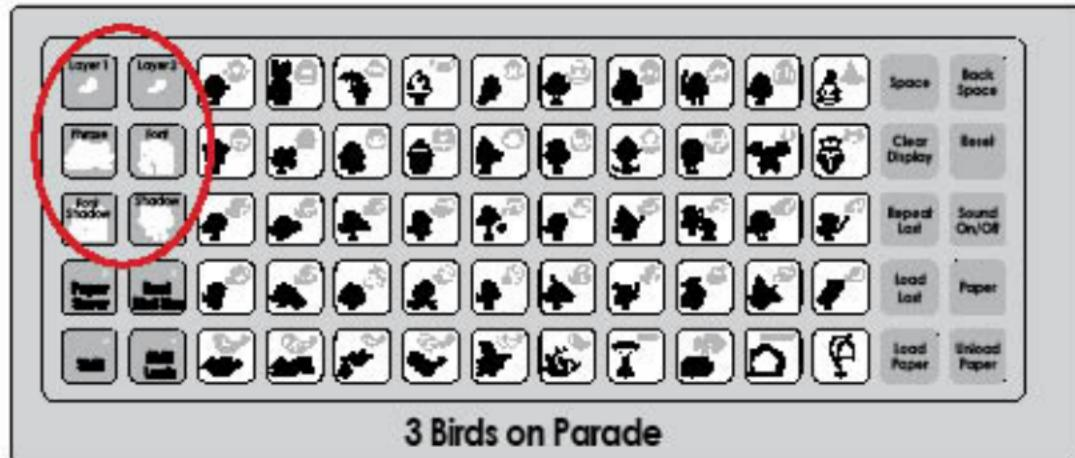
TIP: A Feature can be selected before or after a character has been selected, but before the CUT button is pressed. Once pressed, a Feature key will remain lit until it is turned off in one of the following ways: the Feature key is pressed a second time or the Reset All key is pressed.
