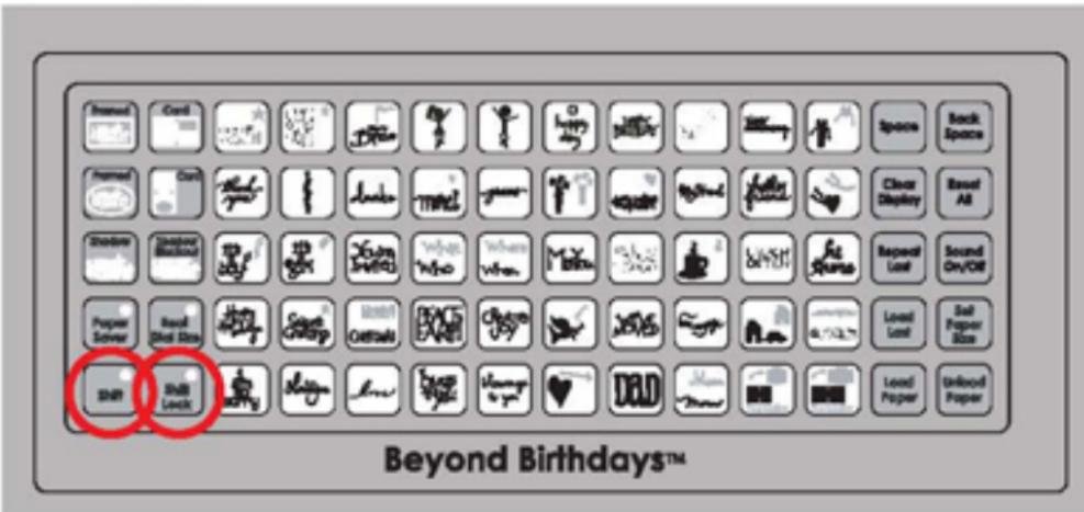
Use the Shift Lock key to select more than one shape or phrase at a time from the upper right corners of keys. Press the Shift Lock key again to deselect it. If a character takes up the entire key , it will be displayed whether Shift is selected or not.
