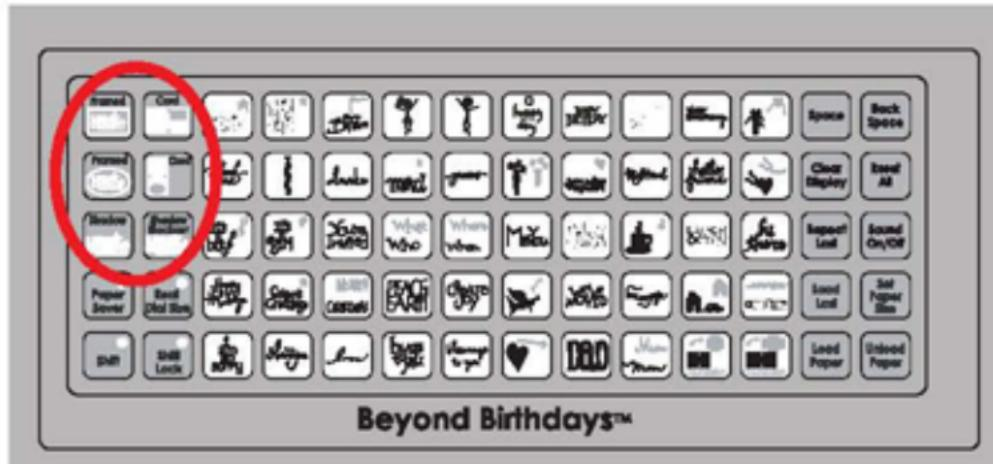
**TIP:** A Feature can be selected before or after a shape or phrase has been selected, but before the CUT button is pressed. Once pressed, a Feature key will remain lit until it is turned off in one of the following ways: the Feature key is pressed a second time, the Reset All key is pressed, or a different Feature is selected. Only one Creative Feature key can be selected for each cut, and that Feature will be applied to all characters on the LCD screen.
