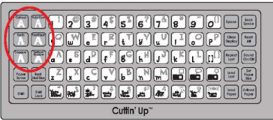
TIP: A Feature can be selected before or after a character has been selected, but before the CUT button is pressed. Once pressed, a Feature key will remain lit until it is turned off in one of the following ways: the Feature key is pressed a second time or the Reset All key is pressed.
