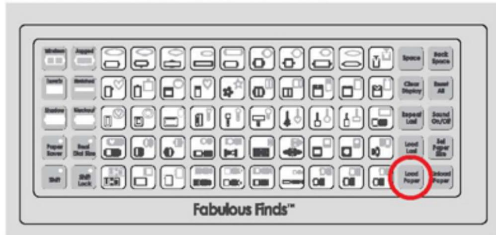
TIP: Your Cricut™ machine needs 12" (30.48 cm) of clear space in the front and back for paper movement in and out of the Cricut™ machine. If your paper does not load correctly, press the **Unload Paper** key and try again.
