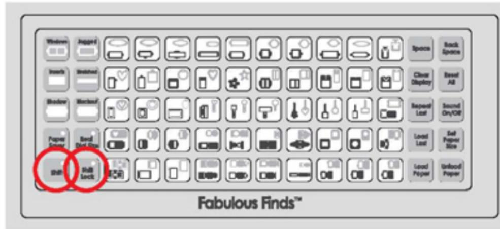
Use the Shift Lock key to select more than one character at a time from the upper right corners of keys. Press the Shift Lock key again to deselect it.
