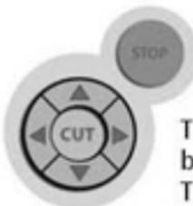
The **STOP** button adjacent to the **CUT** button will stop any operation in progress.
