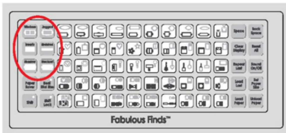
TIP: A Feature can be selected before or after a character has been selected, but before the CUT button is pressed. Once pressed, a Feature key will remain lit until it is turned off in one of the following ways: the Feature key is pressed a second time, the Reset All key is pressed, or a different Feature is selected. Only one Creative Feature key can be selected for each cut, and that Feature will be applied to all characters on the LCD screen.
