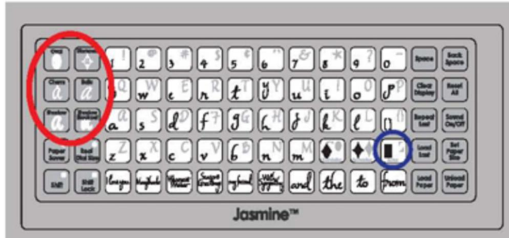
TIP: You cannot mix Features in a cut. Whatever Feature is selected when the CUT button is pressed will determine the look of all the letters, shapes, or phrases on the LCD screen.
