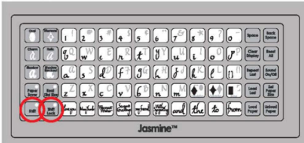
Use the Shift Lock key to select more than one letter, shape, or phrase at a time from the upper right corners of keys. Press the Shift Lock key again to deselect it.
