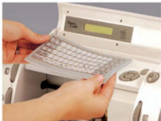
1. Plug in and turn on your machine. Place the Keypad Overlay on the Cricut™ keypad.
