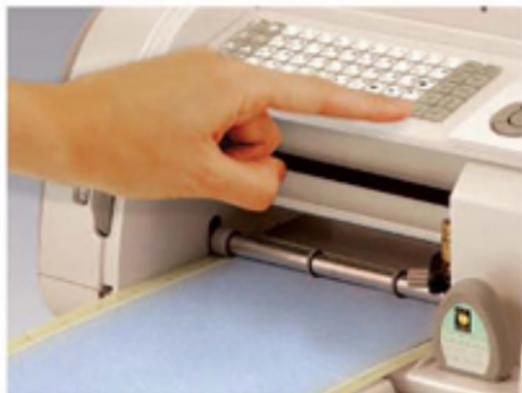
4. Press the **Load Paper** key. The paper will be pulled into the Cricut™ machine.
