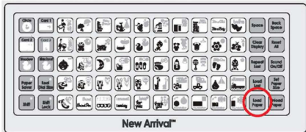
TIP: Your Cricut™ machine needs 12" of clear space in the front and back for paper movement in and out of the Cricut™ machine. If your paper does not load correctly, press the **Unload Paper** key and try again.
