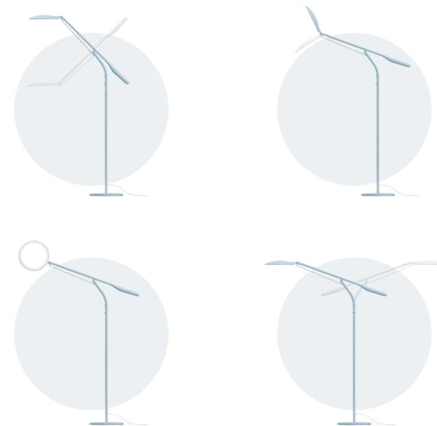
Use lamp head to swivel, pivot & rotate.
