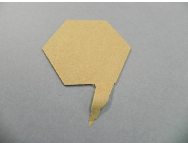
Figure 15: Chipboard, regular, not cut through
