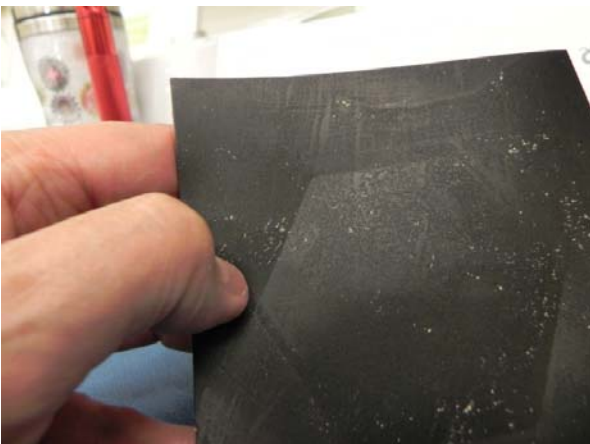
Figure 19: Magnet material not cut through
