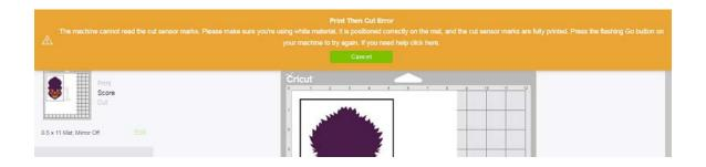
When Design Space tells you that the machine cannot read the cut sensor marks, this means that the image that you are trying to cut is set to Print then Cut. The machine is searching for the cut sensor marks that will allow it to cut the image accurately. If you did not intent to Print then Cut, and would rather cut only, you can easily change your image's line type from a Print line type to a Cut line type. Follow the instructions found here to change the image line type.
