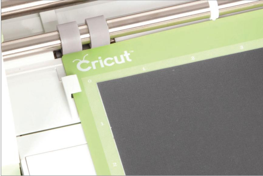
**Step 3** Keeping the mat pressed firmly against the rollers, press the flashing Load/Unload button on the machine.
